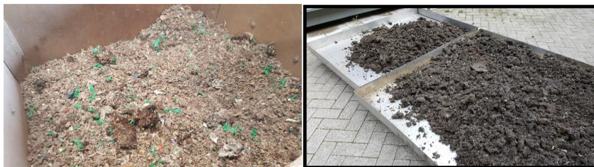
Figure 13. Pre-treatment reject from REG on left side and solids bio-residues from biogas reactors (digestate) on right side.
