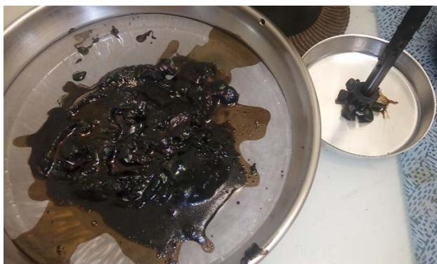
Figure 8. Picture of bio-crude directly poured on a metallic sieve for aqueous phase separation, on the right reactor stirrer after the experiment, W2R 10, test on kraft black liquor at 300°C.
