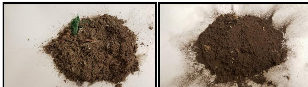
Figure 14. Pre-treatment reject (left) and digestate (right) after drying and grinding.
