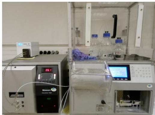
Figure 11. Picture of the GPC Malvern system GPC-Max / TDA
