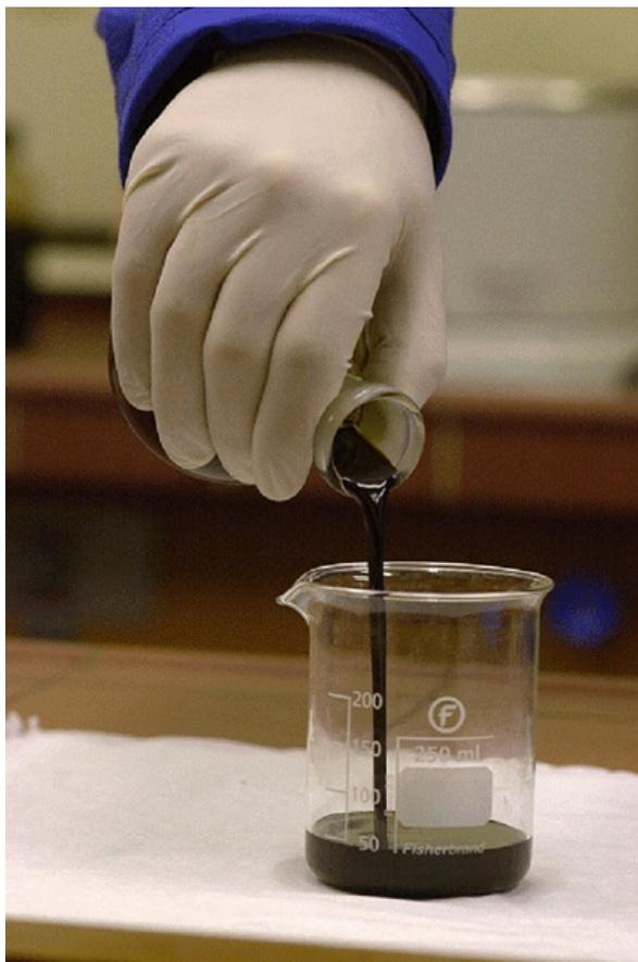
Figure 2: Picture of a typical FPBO from woody biomass.
