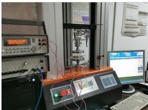
Set-up in UPT ICR measurement
