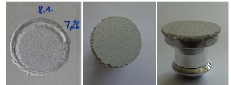
Adhesion failure close to the metal coating interface for all specimen 14
