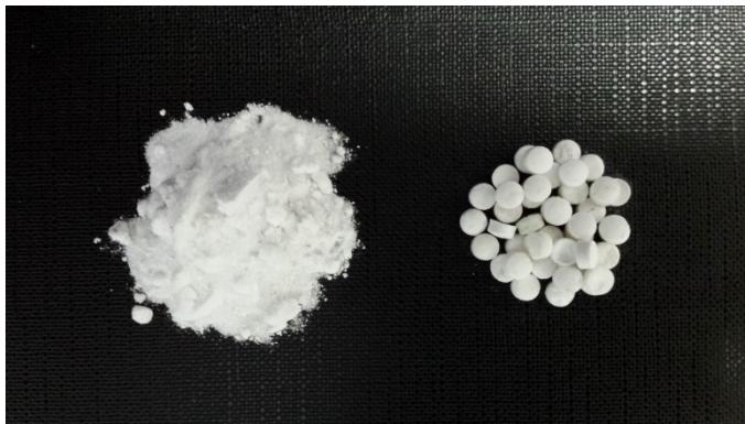
*~1 g amounts of MCF-PEI80b before (left) and after (right) shaping via SPTP<sup>1</sup>.*
