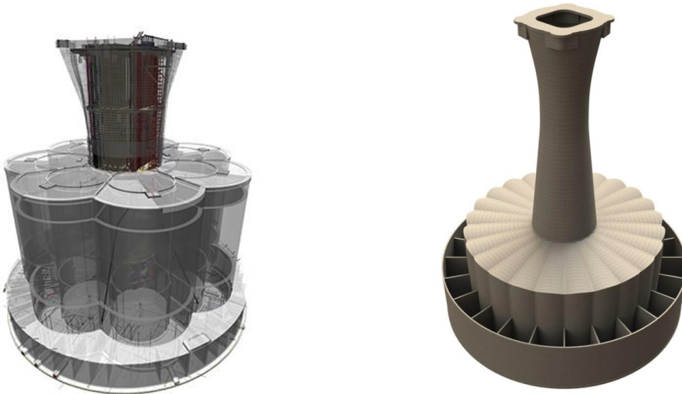
Figure E2. Offshore gravity base concrete structures:
