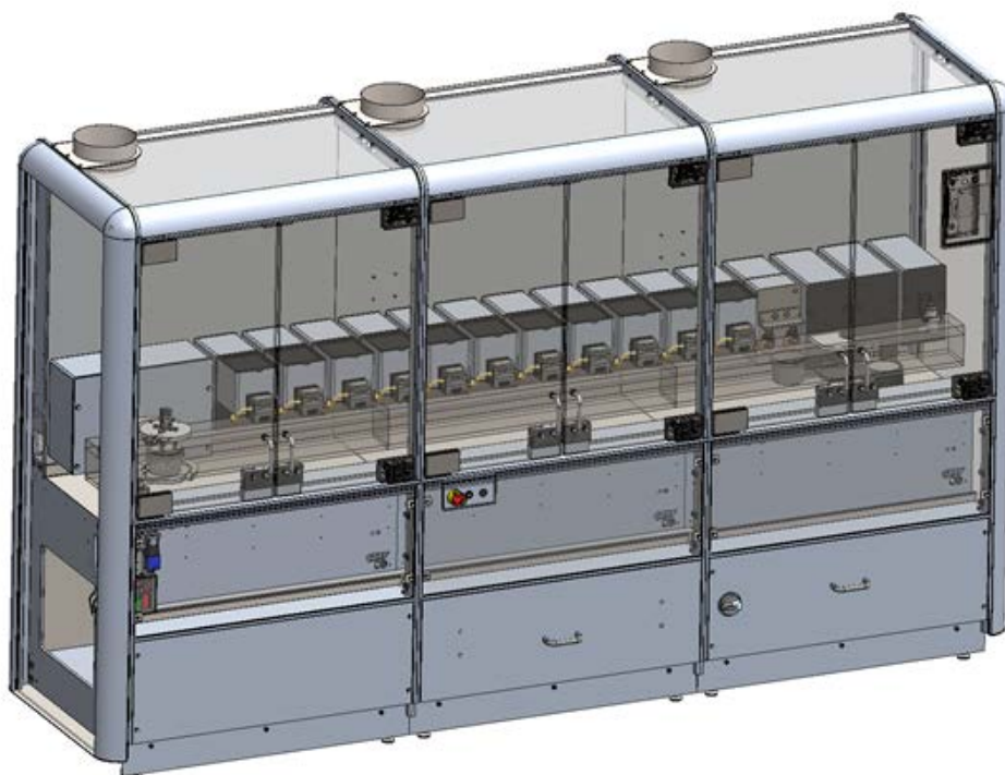
Figure 1 displays the CAD-model of the FabLab with all the different modules for liquids installed.
