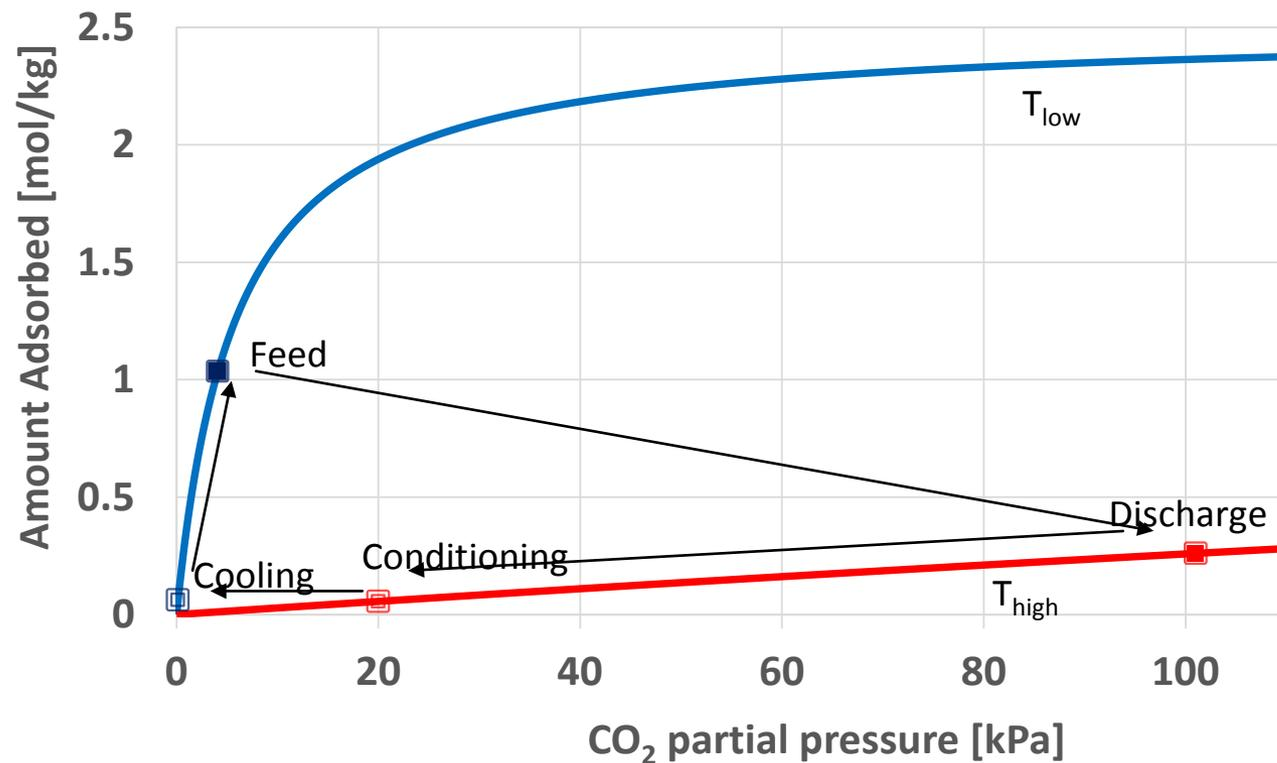
Adsorbent will remove CO<sub>2</sub> from flue gas at a lower temperature and then heated to desorb it. Other conditioning steps should be made followed by a cooling to restore the unit to a new cycle
