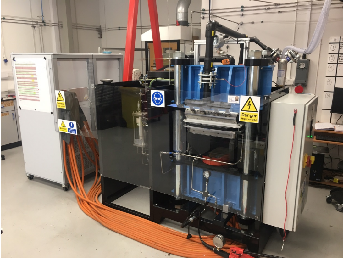
Figure 3: Completed prototype electrolyzer system.
