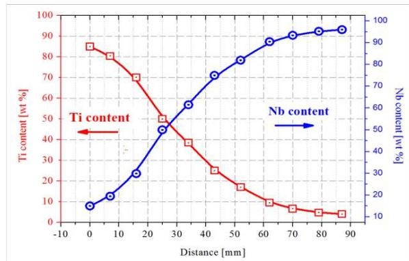
Compositional spread in the Ti-Nb system manufactured by magnetron sputtering out of elemental targets
