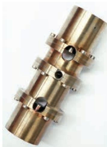
Pulse-echo speed of sound cell at Ruhr-Universität Bochum. (Photo: RUB)
