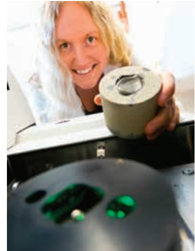
SINTEF scientist Malin Torsæter is using micro computed tomography to investigate the interior of a sample consisting of cement and rock. (Photo: Thor Nielsen/SINTEF)
