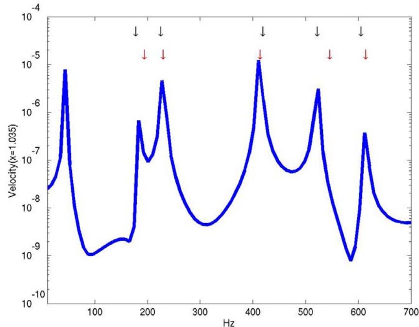
Cold flow simulations give good fit between resonant frequencies for experimental (black arrows), linear simulation (red arrows) and non-linear simulation (blue line) results
