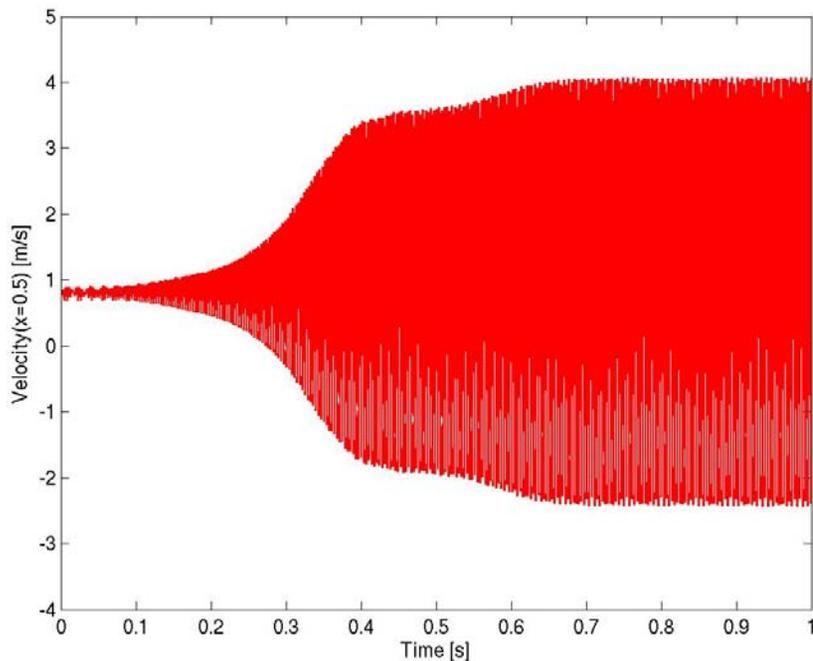
Envelope of velocity at single point in premixer for various reflection parameters. The red line is the envelope of the left plot
