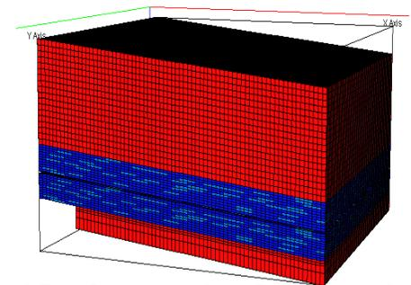
**3D view and gridding of the model containing two overburden blocks shale and sand body patches**
