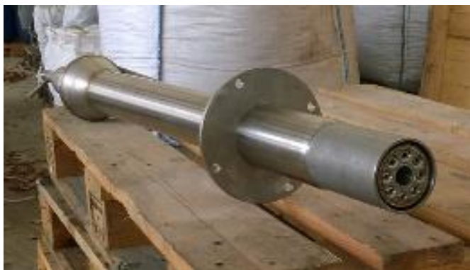
Oxyfuel burner design by ThyssenKrupp for cement plant operating conditions
