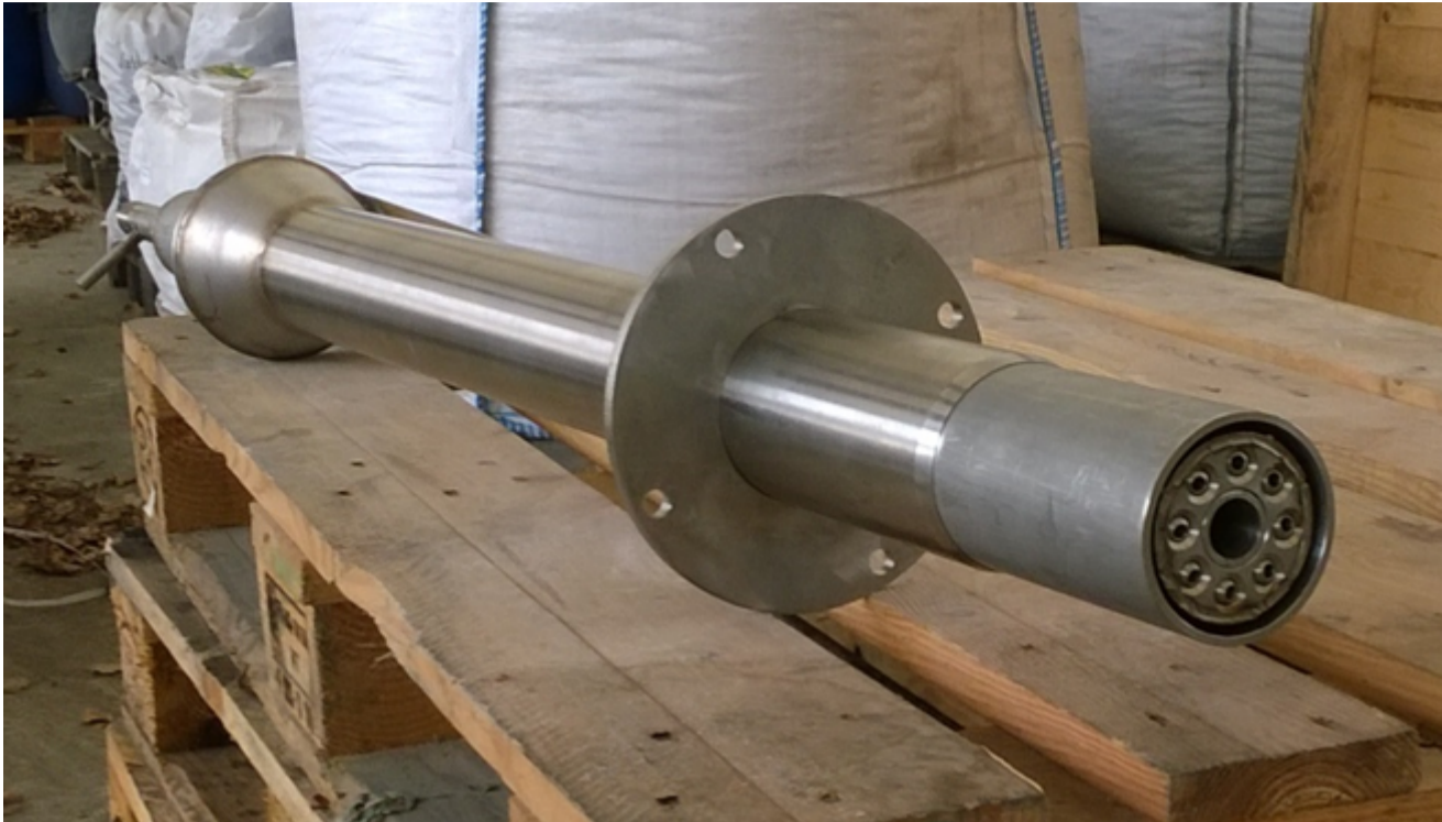
An oxyfuel burner
