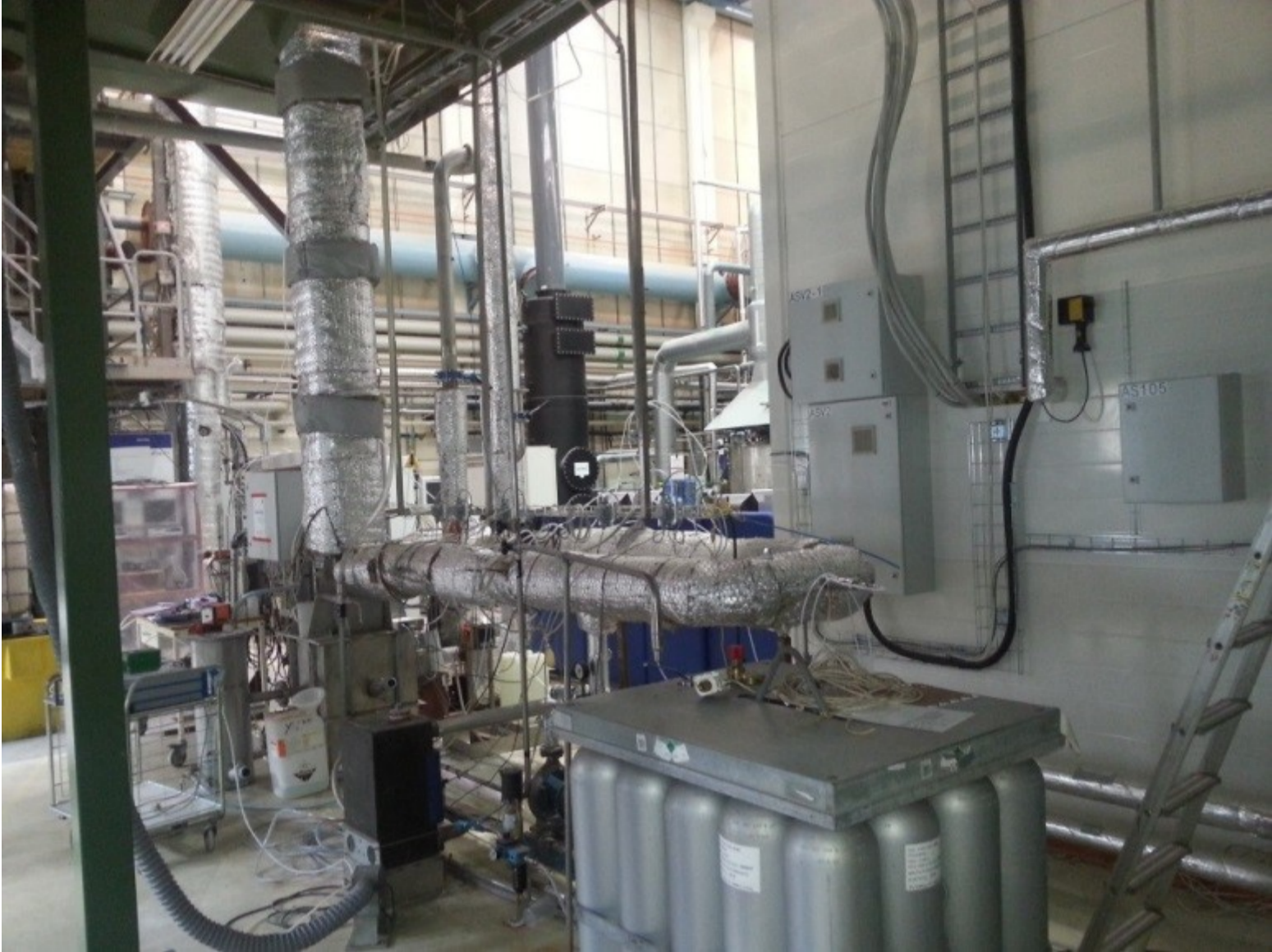
Experimental rig used for the Direct Contact Cooler (DCC) tests carried out by GE Power Sweden.
