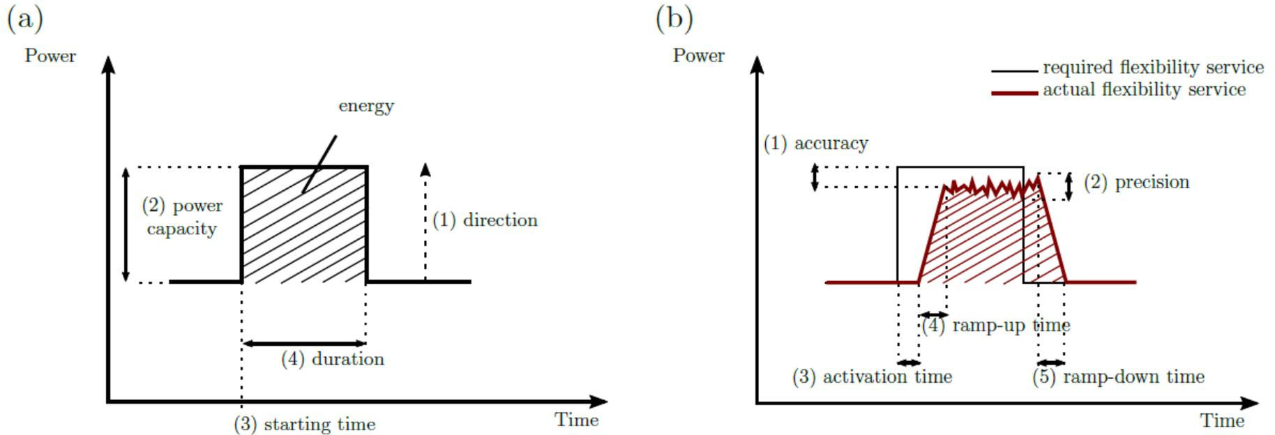
Figure 1: (a) Theoretical and (b) practical attributes of a flexibility service (excluding the location).
