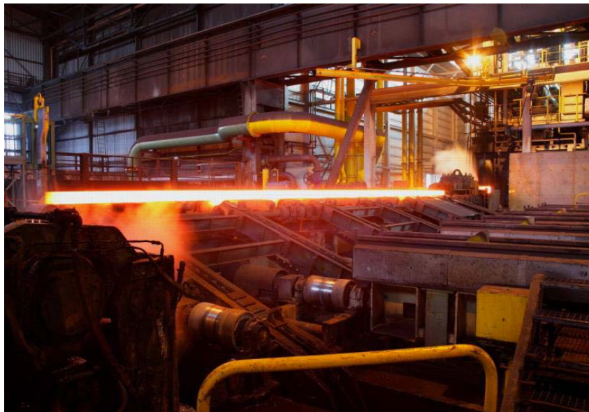
Figure 4: A hot, glowing bar in the Saarstahl rolling mill
