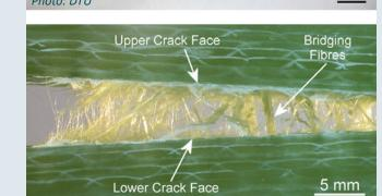
Fracture process zonelarge-scale crack bridging in composites
