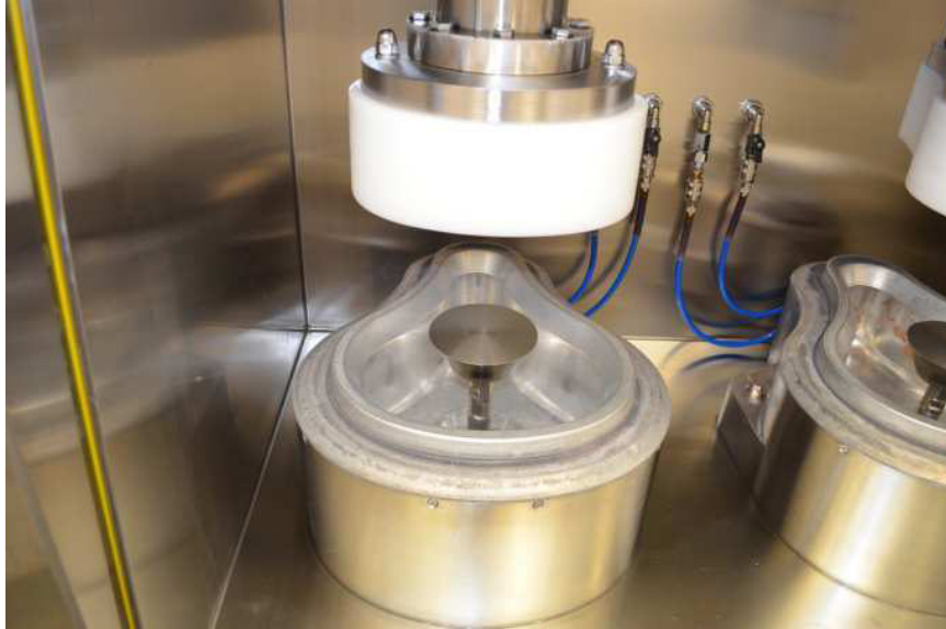
Figure 2: Pressing device for final shape of ham
