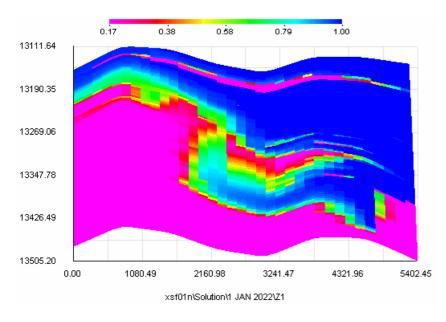
CO<sub>2</sub> saturation in fine scale vertical slice of flow simulation model
