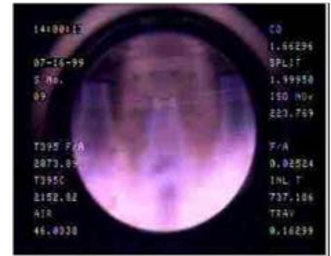
F-class H 2 Combustion Validation ... Video Capture of Flame Structure 85-90% H 2
