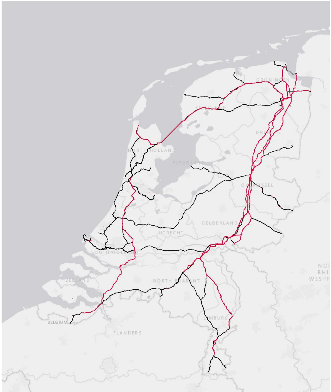
Figure 5.11: A map with the natural gas and hydrogen backbone of Gasunie. In black , the existing gas backbone (only pipes shown with a diameter of 24 inch or more). In red , the incomplete hydrogen backbone as proposed by Gasunie (only pipes shown with a diameter of 48 inch). The hydrogen backbone can be realised by converting the parallel low calorific natural gas infrastructure to hydrogen infrastructure. Interrupted routes are to be completed by Gasunie and are within the scope of the hydrogen backbone.
