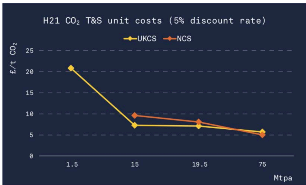
Figure 6-2 Summary H21 unit transport and storage cost estimates per tonne CO 2 – all UK Continental Shelf and Norwegian Continental Shelf cases 110
