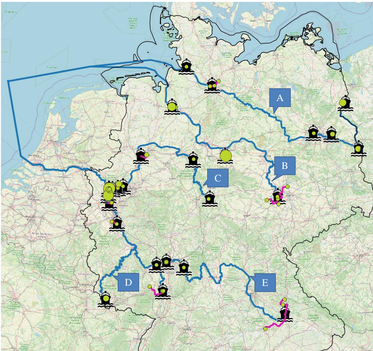
Figure 2.10: Water transport routes (blue), remaining CO 2 sources (green), loading stations (black symbols) and CO 2 pipelines (pink). Map in background © OpenStreetMap contributors
