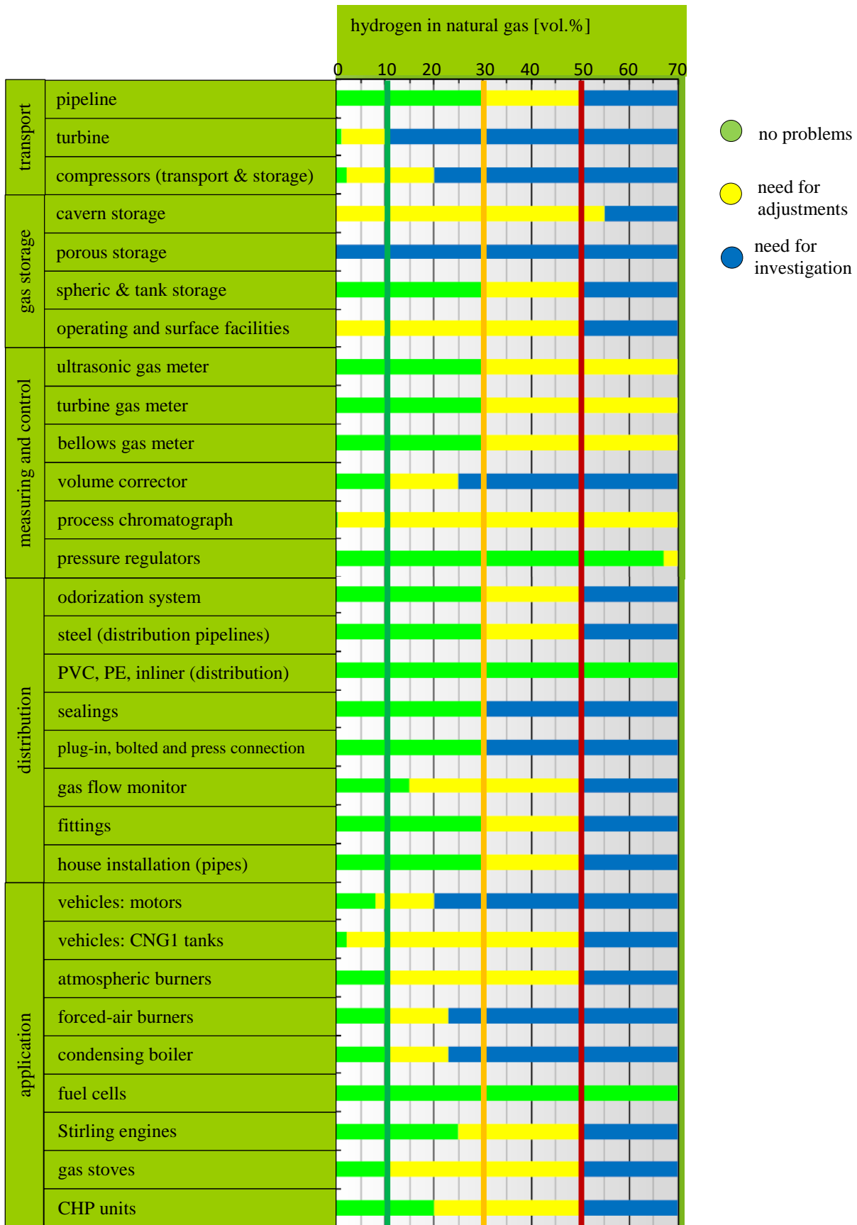
Figure 2.11: Hydrogen compatibility of natural gas infrastructure assets – taken, translated, and slightly modified from [DVG13]
