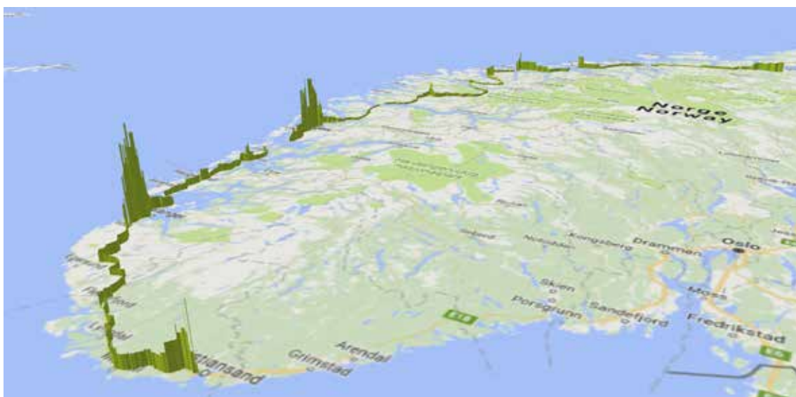
Figure 12 AADT along E39. The height of each profile is determined by the AADT from NVDB.
