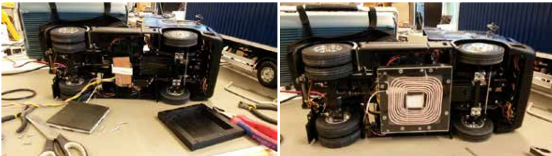
Fig. 8 Assembly of the on-board coil and associated resonant capacitors on the truck model.
