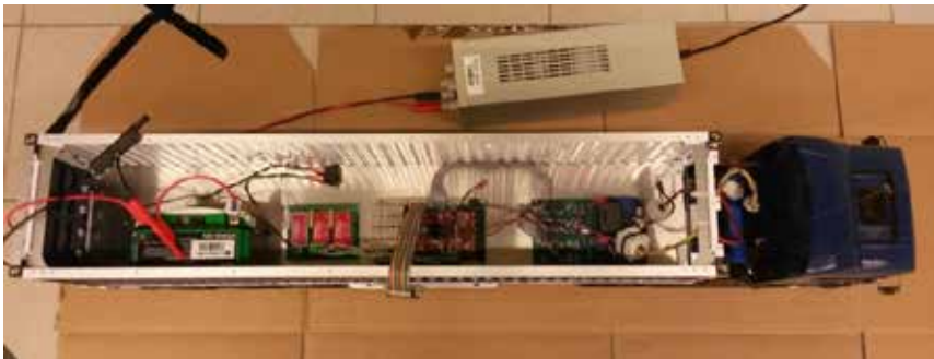
Fig. 11 On-board power conversion system for the IPT, including battery, H-bridge and controls.
