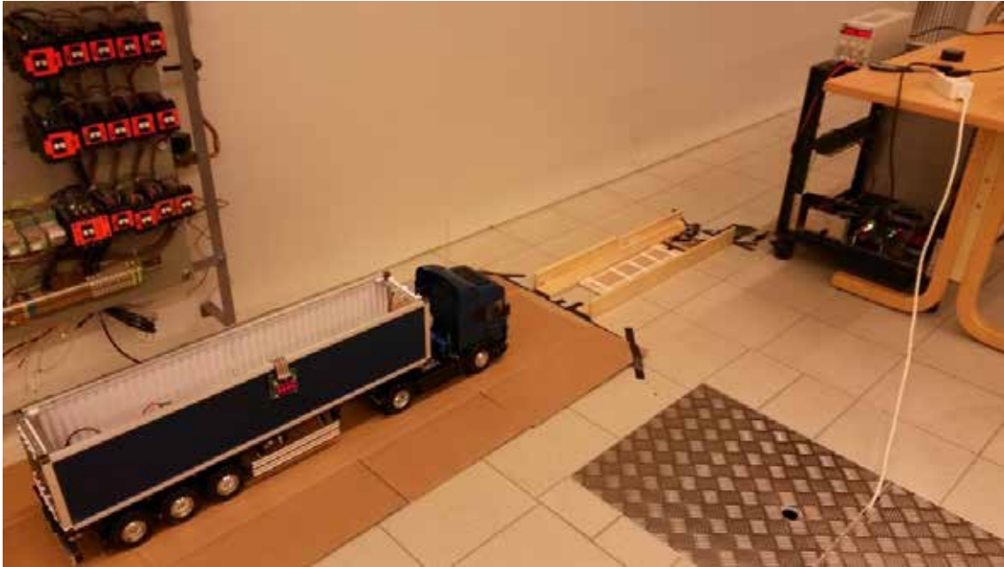
Fig. 13 The radio-controlled truck model running on the on-road coil, demonstrating the dynamic inductive power transfer
