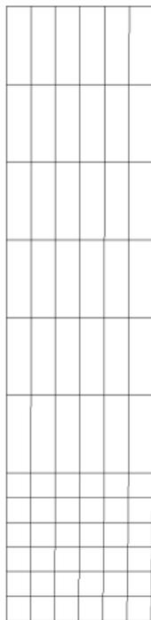
a) Mesh for one quadrant of the strip with 6 knot spans in the width and 12 in length  $\Rightarrow 7 \times 13$  grid points (basis functions)
