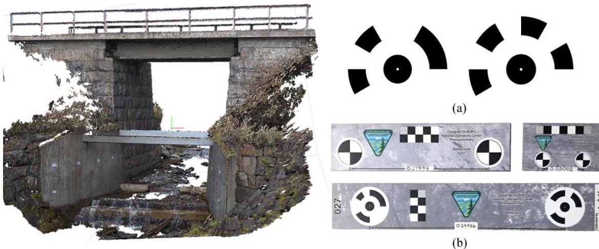
Figure 33. Ground-based photogrammetry camera for Juvajokk Bridge (left), artificial targets used in the alignment process and for scaling: (a) coded targets and (b) calibration scale bars (Popescu et al., 2019b)
