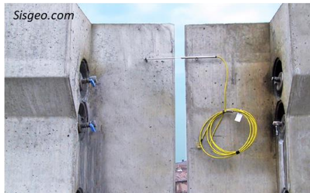
Figure 54: Left: Working principle of LVDT sensor (learnmech.com) and an example of a commercial sensor (bditest.com). Right: Example of LVDT installation to measure displacement between two structural parts (sisgeo.com)
