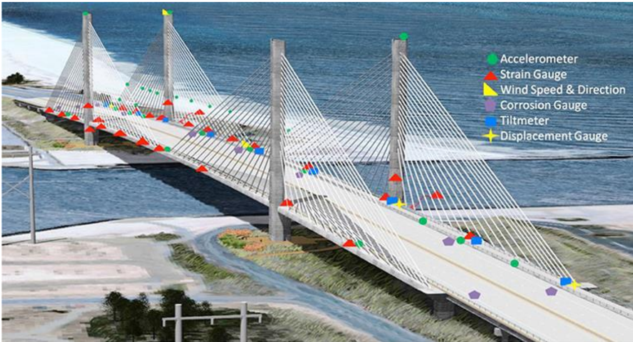
Figure 50: Example of structural health monitoring of a cable-stayed bridge (Al-Khateeb et al., 2019)
