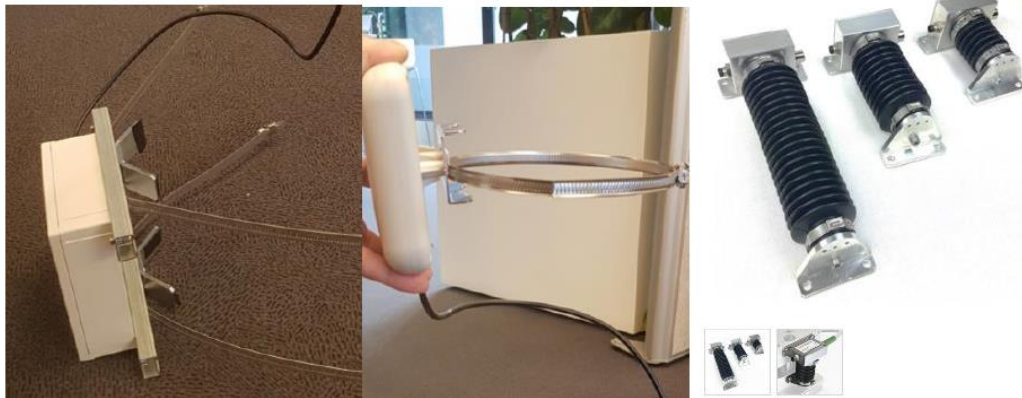
Figure 79: Accelerometers with battery package from the monitoring (left and middle) and distance measuring device (right); ( www. Lisab.se/product/eds-series/ )
