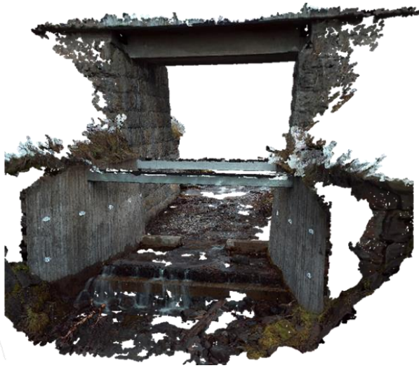
Figure 21: Infrared scanning using Matterport Pro2 camera for Juvajokk Bridge (Popescu et al., 2019b)
