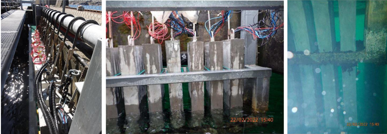
Figure 84: Instrumented concrete beams exposed to tidal water at Austefjord Field Station, Bergen (Foto: Andres Belda Revert 2021)
