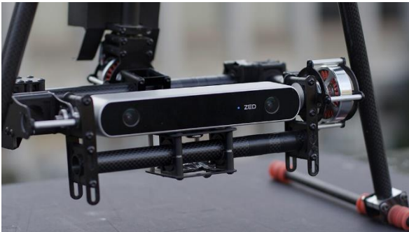
Figure 29: ZED 2K Stereo Camera from Sterolabs ( https://thenextweb.com on 2023-10-01)
