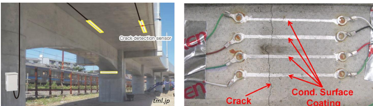
Figure 61: working principle of conductive surface sensors (left, tml.jp) and example of crack detection by installation of conductive paint (Raoufi et al., 2011).
