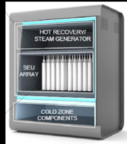
SEUs integration in hot box with required ancillary equipments
