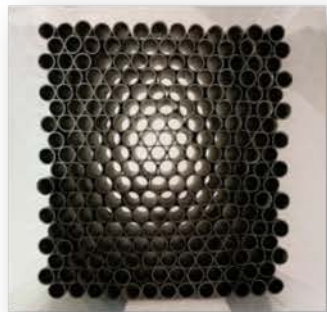
Tubular cells (electrodes, electrolyte, current collectors)
