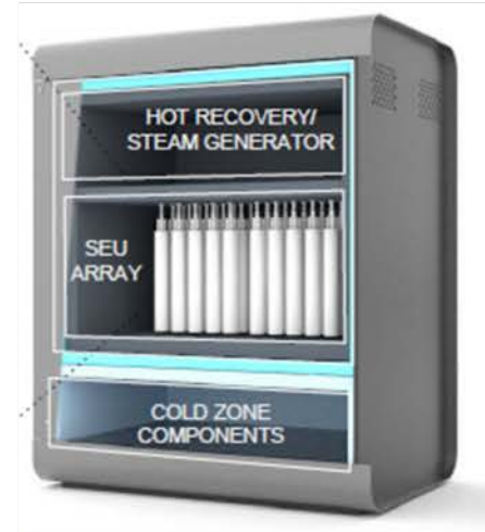
SEUs integration in hot box with required ancillary equipments
