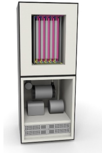
SEU integration in hot box with required ancillary equipment
