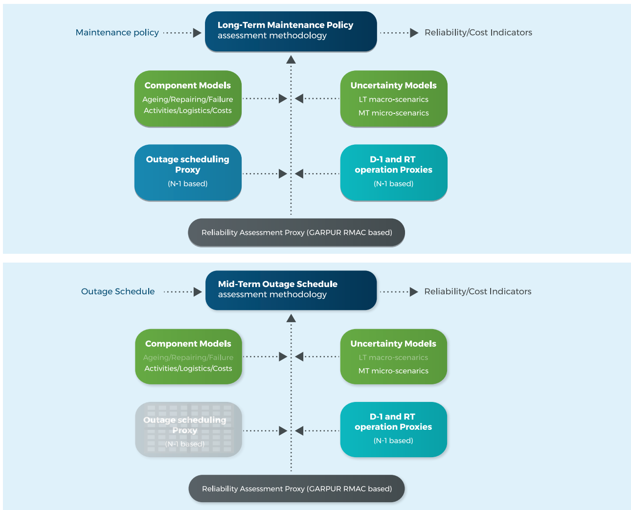
Schematic representations of the assessment proposals for maintenance policy and outage scheduling highlighting the methodology and the use of shorter-term proxies.
