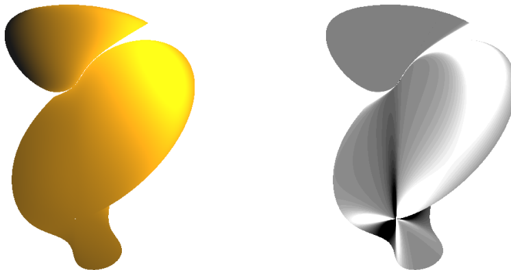
Fig. 1.5. A quartic surface where all first order derivatives vanish, leading to a breakdown in the lighting equation (which is based on calculating the normal by taking the cross product of derivatives). This breakdown is clearly visible in the left image, where the shape looks flat and uninteresting. The right image shows the curvature field, clearly depicting the singularity which is invisible in the first image.
