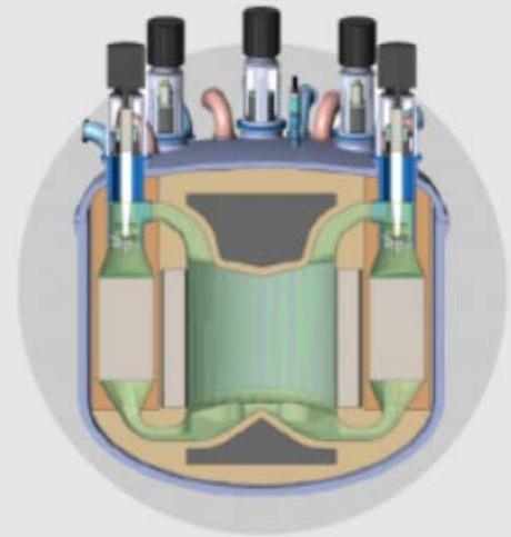
**Molten Chloride Fast Reactor**
