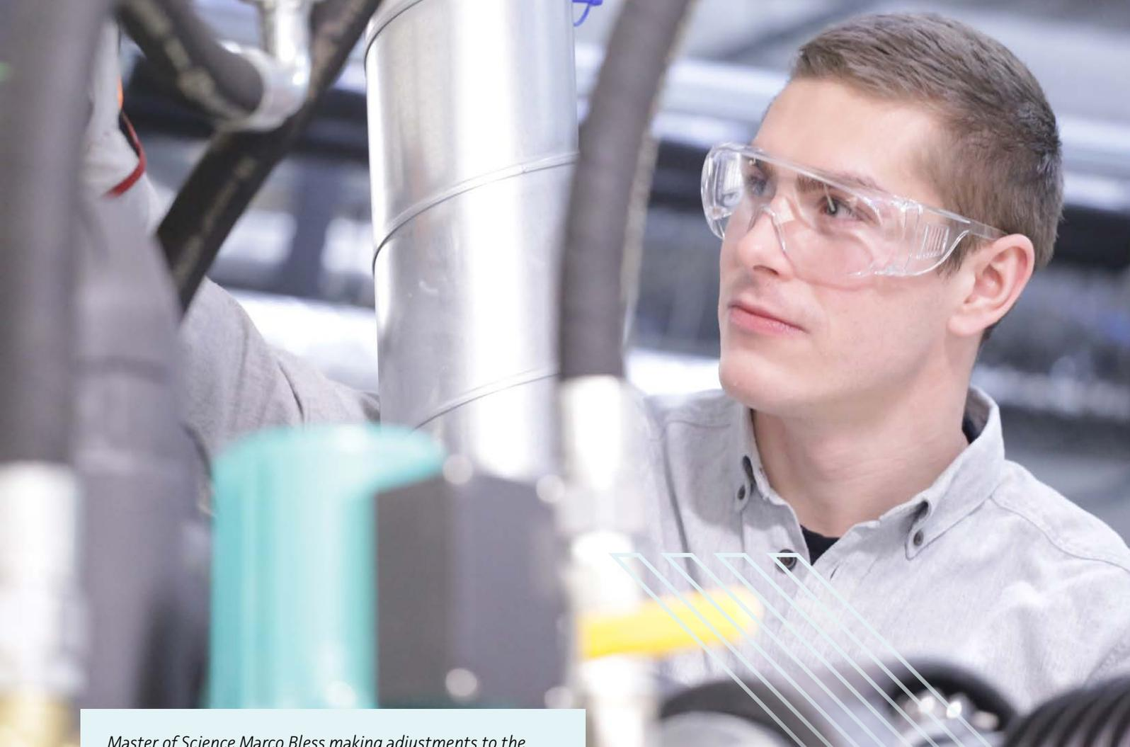
*Master of Science Marco Bless making adjustments to the propane-butane high-temperature heat pump at HighEFFLab.*
