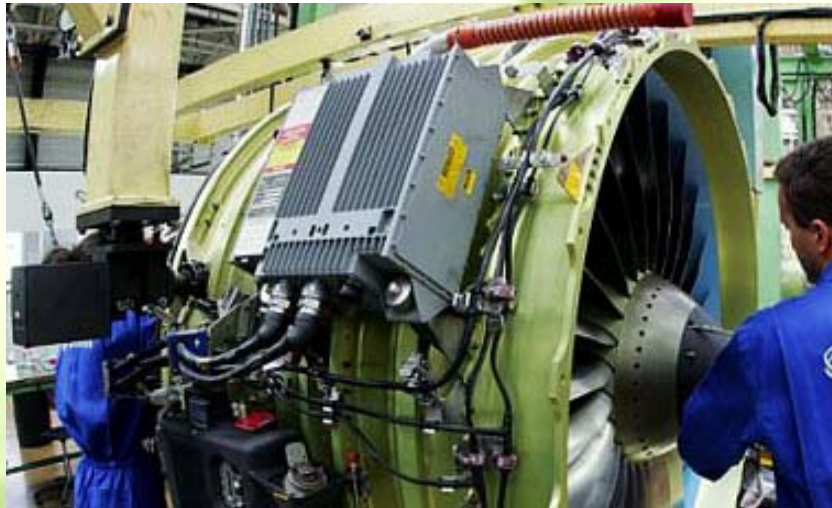
Today's FADEC (Engine Control Unit)
