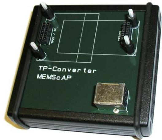
Figure 1 – TP to USB converter
