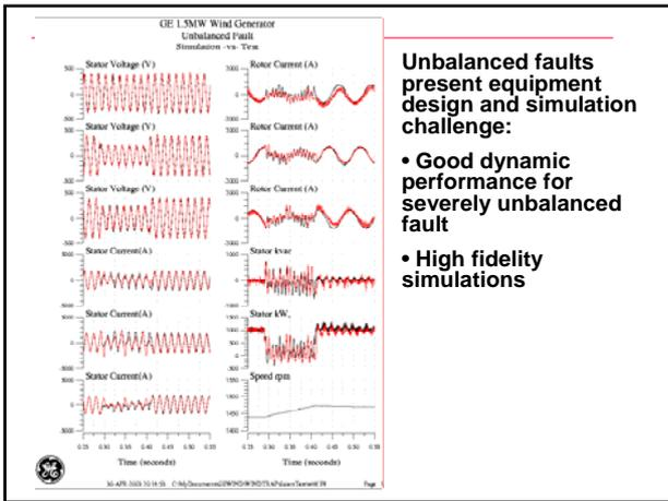
**Unbalanced faults present equipment design and simulation challenge:**
