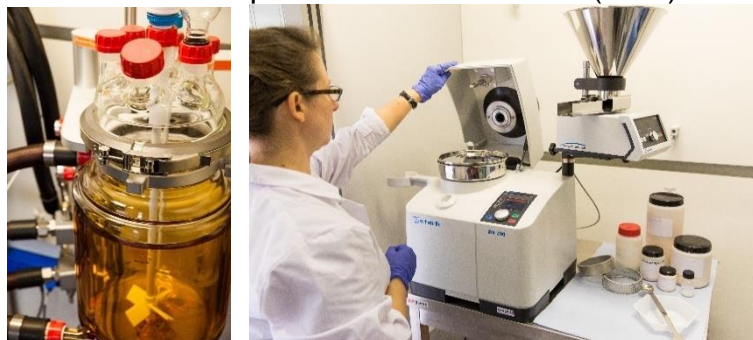
Figure 2: Pictures of the 15 L reactor at ChemStream for making SAPs and the RETSCH ultra centrifugal mill ZM200 for grinding the SAPs to powders
