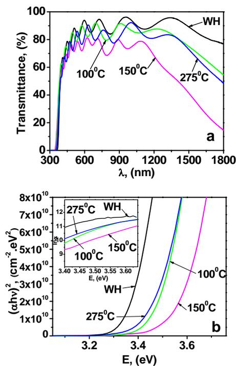
**Figure 2** Dependence of the transmittance of the wave length (a) and of the absorption coefficient as a product  $(\alpha \cdot h\nu)^2$  on energy (b) of ZnO:V thin film deposited at different substrate temperatures.
