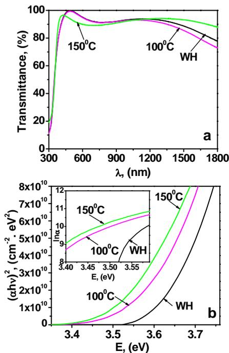
**Figure 1** Dependence of the transmittance of the wavelength (a) and of the absorption coefficient as a product  $(\alpha \cdot h\nu)^2$  on energy (b) of ZnO:Al thin film deposited at different substrate temperatures.
