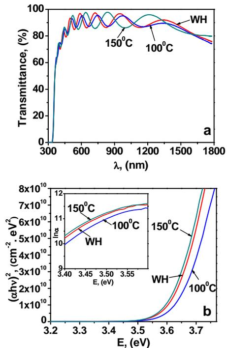
**Figure 3** Dependence of the transmittance of the wave length (a) and of the absorption coefficient as a product  $(\alpha \cdot h\nu)^2$  on energy (b) of ZnO:Nb thin film deposited at different substrate temperatures.
