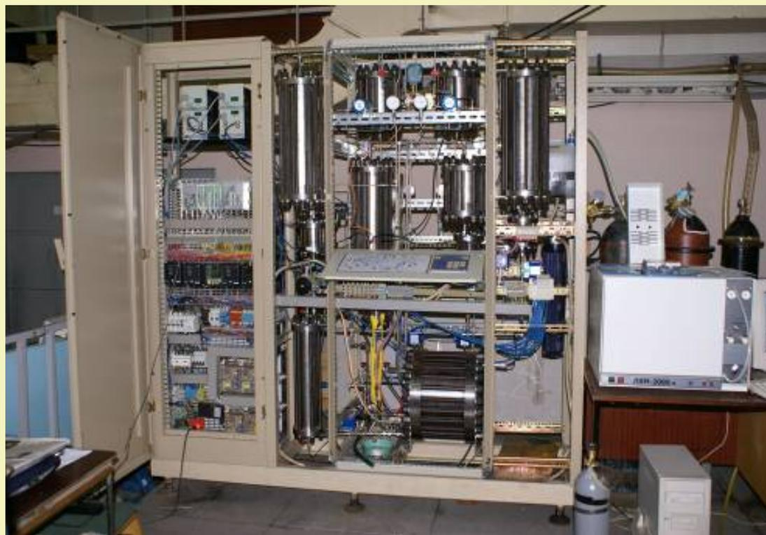
130 bar PEM electrolyzer test station
