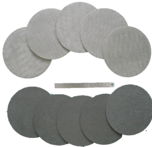
150 cm 2 optimized current collectors for 5 cell stack
