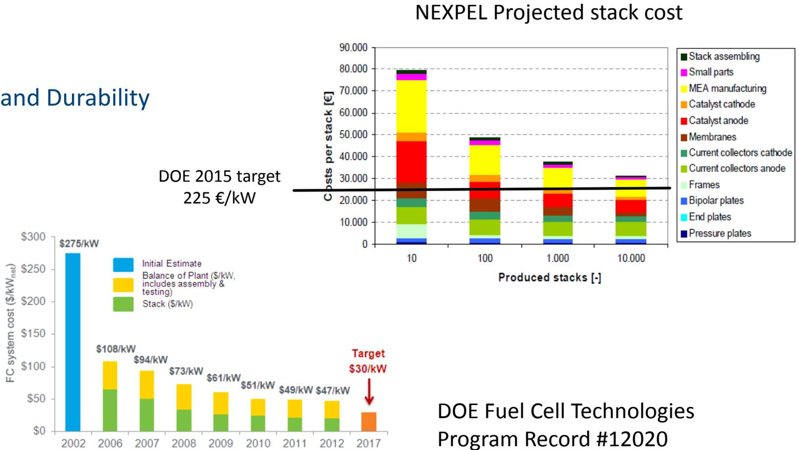
Figure 1. Modeled cost of an 80-kW<sub>net</sub> PEM fuel cell system based on projection to high-volume manufacturing (500,000 units/year).
