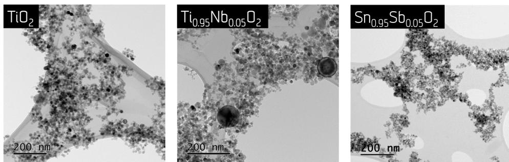
Figure 1: TEM micrographs indicating morphology and crystallite-/particle size.
