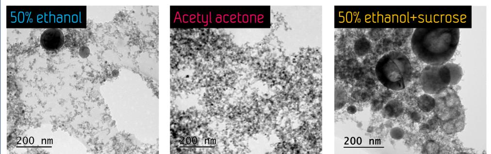
Figure 3: TEM micrographs indicating the effect of precursor solutions on powder morphology and crystallite-/particle size.
