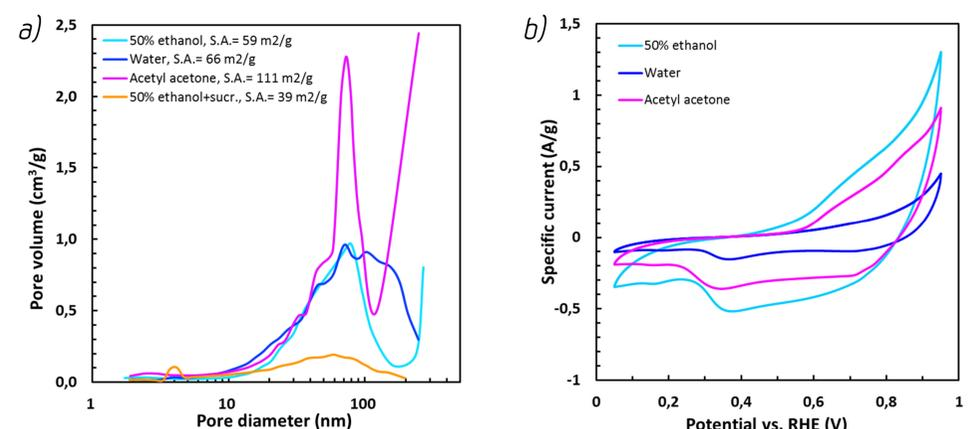
Figure 5: a) Pore size distribution and BET surface area from nitrogen adsorption/desorption measurement. b) Voltammograms: effect of synthesis route on performance.
