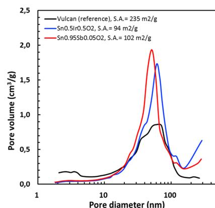
Figure 2: Pore distribution in SnO<sub>2</sub>-powders.
