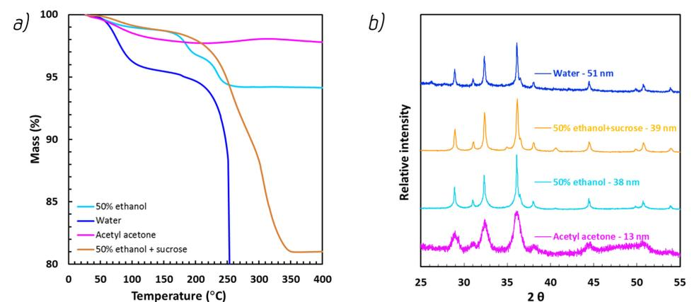
Figure 4: a) TGA and b) XRD indicating degree of combustion/crystallization.
