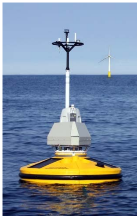
Figure 5 The FUGRO LIDAR based met-ocean buoy (left). Integrated simulations of semi-submersible offshore wind turbines with NOWITECH developed software performed well in the international comparison IEA Annex 30 OC4 (right).
