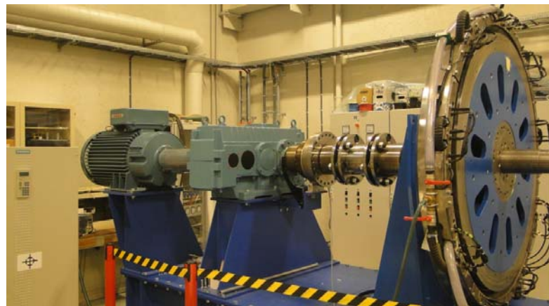
Figure 7 Lab setup with ironless permanent magnet machine.
