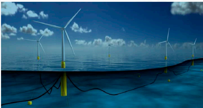
Figure 1: Statoil is now taking the floating wind turbine concept, Hywind, to the next step with a 30 MW pilot wind farm to be installed in Scotland in 2017. Ill: Statoil.
