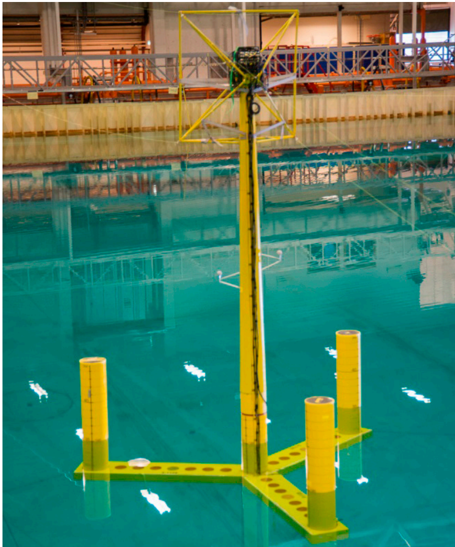
Figure 8: Scaled HIL model test of an optimized floating wind turbine. Photo: MARINTEK.
