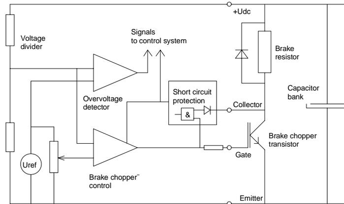
This board monitors the DC-link voltage, and controls an IGBT brake chopper. Overvoltage trip setpoint is determined by a voltage divider. Default trip level is 640V. Brake chopper operating voltage is adjustable between 0%-100% of overvoltage trip level.
