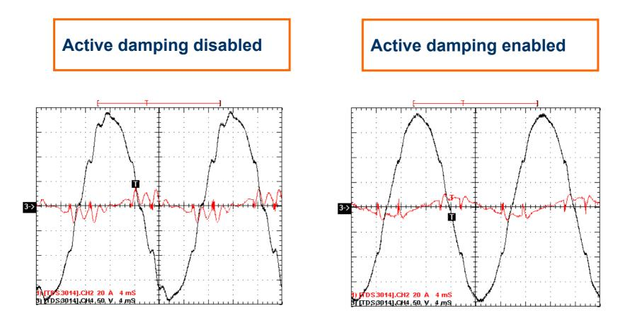
voltage at bus A (black)current C (supply line) (red)
