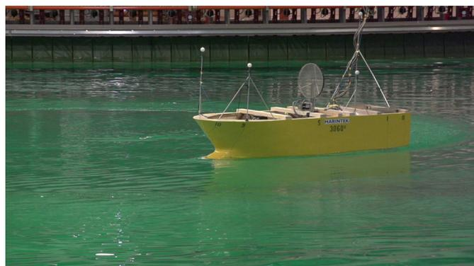
Figure 2. Free sailing tests with model of R/V Gunnerus.
