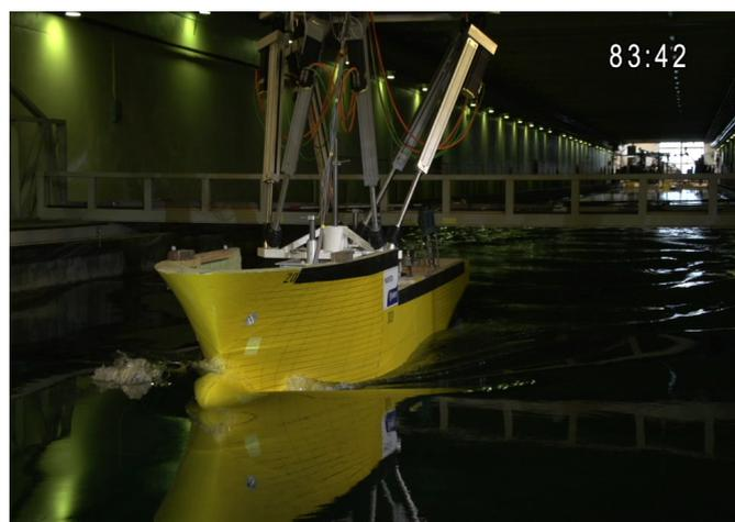
Figure 3. PMM model tests of Island Condor.
