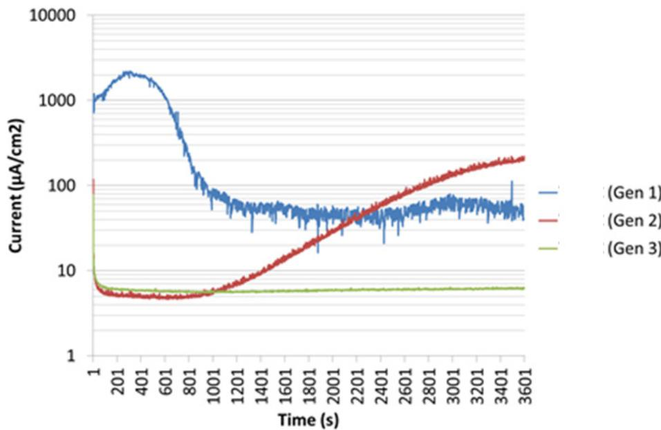
**Figure 1: Potentiostatic corrosion tests at 1.4V for three generations of a PVD coating.**
