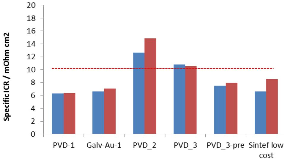
**Figure 6: Specific ICR @ 166 N cm<sup>-2</sup> (land area 6.19 cm<sup>2</sup>), before and after AST.**
