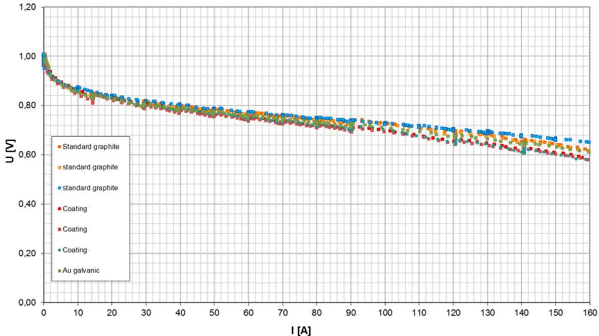
**Figure 9: Current voltage curves of the cells with the different coated bipolar plates.**
