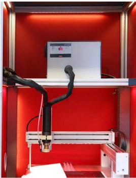
*Atmospheric pressure steam and air plasma cleaning prototype by Fronius.*
