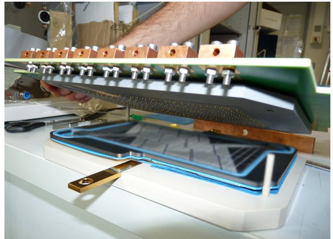
A segmented, automotive size graphitic test cell (LxWxH= 300x150x2 mm) and cell housing with compression unit and electrical cell contacts for the integration of the segmented cell.
