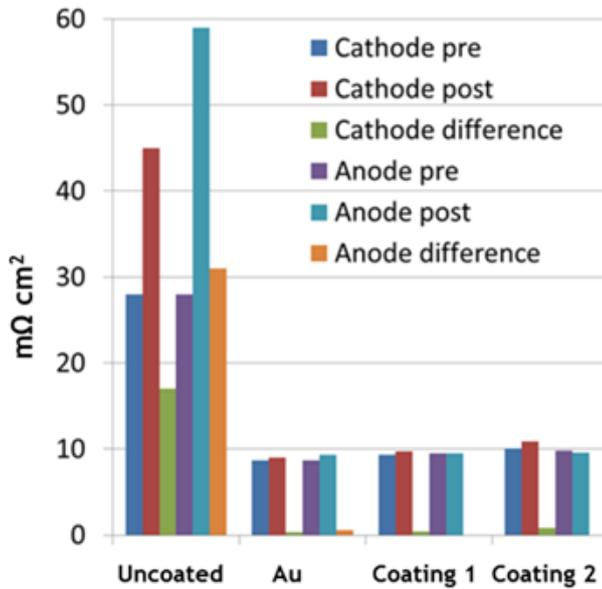
Status of best coatings after small scale in-situ AST, 100 hours cycling between OCV and 0.4 V.
