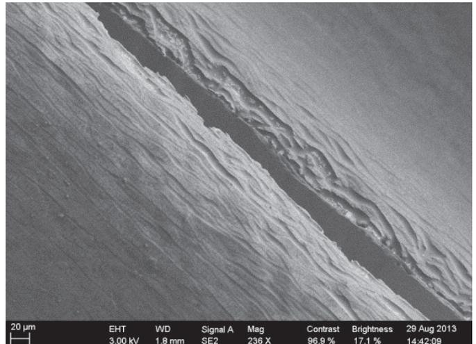
*Stamping of pre-coated plates, where the coating still adheres but cracks when the metal is stretched up to the elongation limits.*
