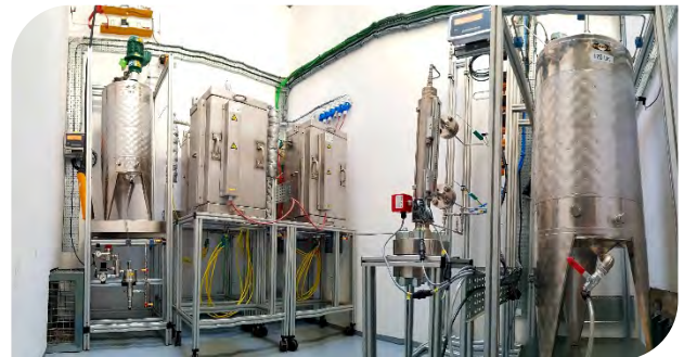
BTG's 50 kg/day hydrotreater (4-6 L catalyst)
